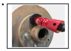
Place the wheel hub cleaning tool over a wheel mounting stud and start the impact wrench to clean away rust and corrosion from the hub. Repeat this process for additional studs requiring cleaning/resurfacing.
