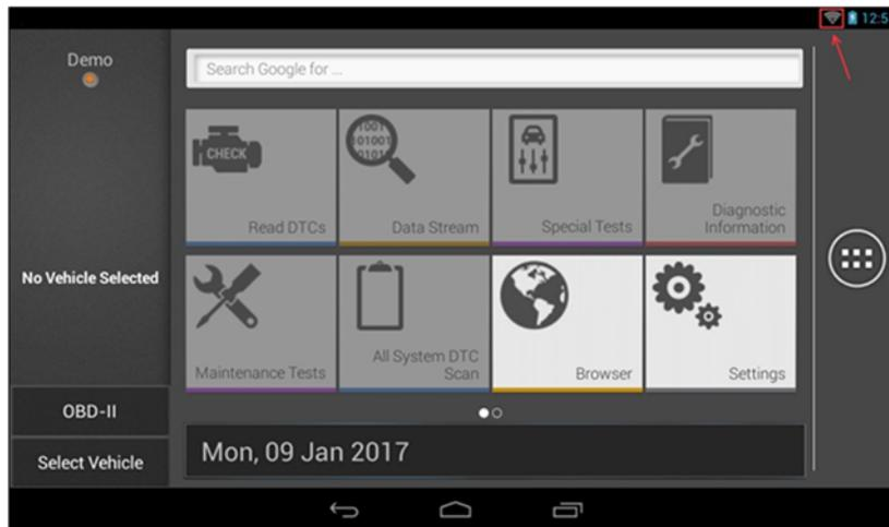
2. Connect to a vehicle and access the Diagnostics Report that you want to Print (currently available from Read DTCs, All System DTC Scan or Automated System Test) and locate the **Share** option
